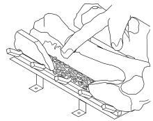
Figure 58 - Placing Ember Material on Burner
